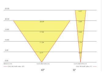
In lighting, choosing the lens angle is as important as selecting the color or wattage. Small angles retain brightness at long distances, while wide angles cover larger areas but lose brightness over distance.
